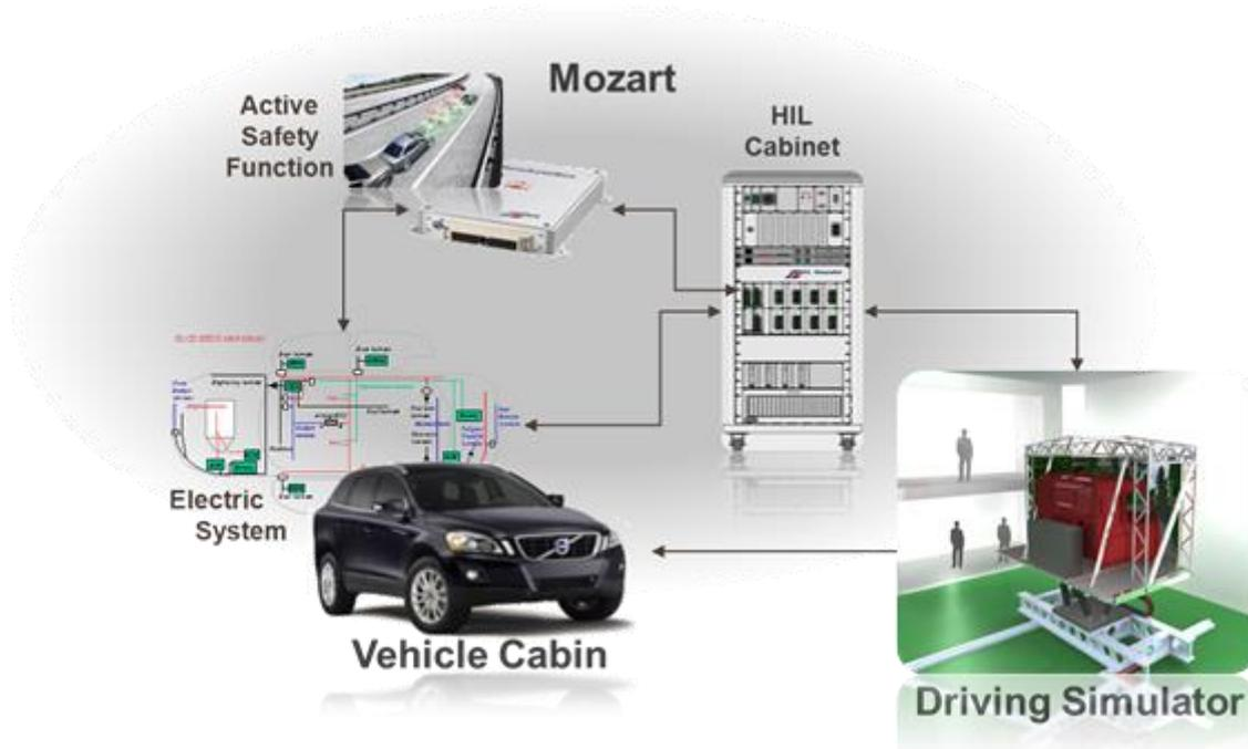
Figure 1. Integrated test environment for active safety functions utilizing an advanced driving simulator.
