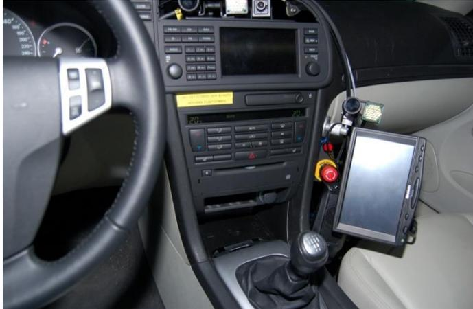
Figure 6. Position of the display presenting the visual distraction task (note that the picture is from another simulator than Sim IV). (Photo: Mikael Ljung Aust).
