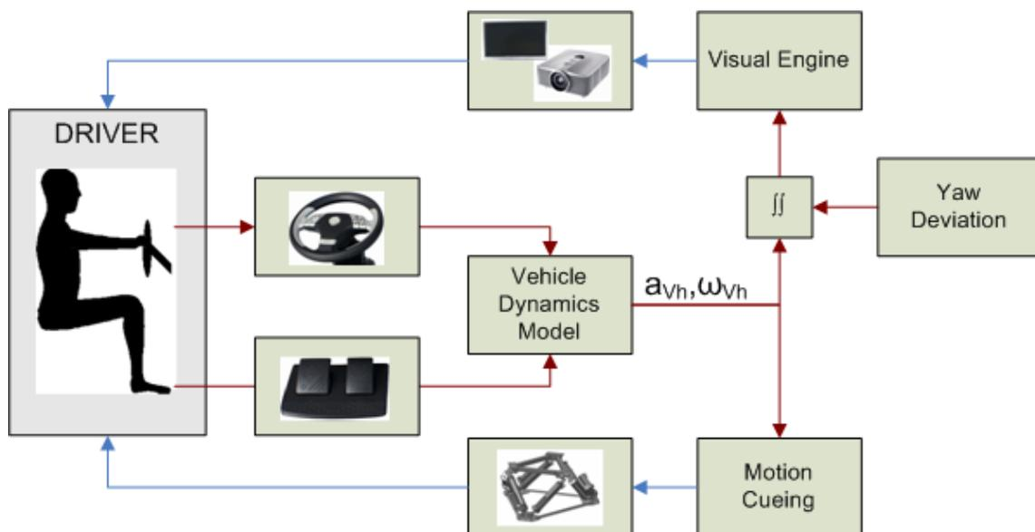
Figure 7. Driving feedback loop with interfering yaw deviation function.
