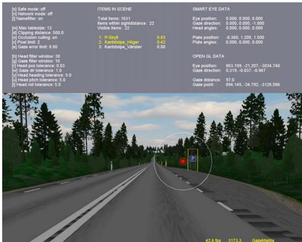
Figure 2. Screen shot from a prototype able to visualize the driver's gaze in the simulator graphics (Nordenrot, 2009).
